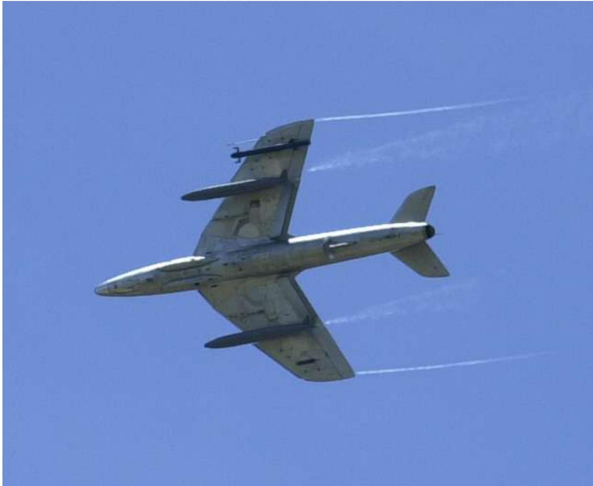
*Returning after my first Hunter flight in 45 years. Fuel can be seen trailing from the drop tanks trying to fall off, with the moderately high 'g' break. The maintenance was not nearly up to military standards.*
