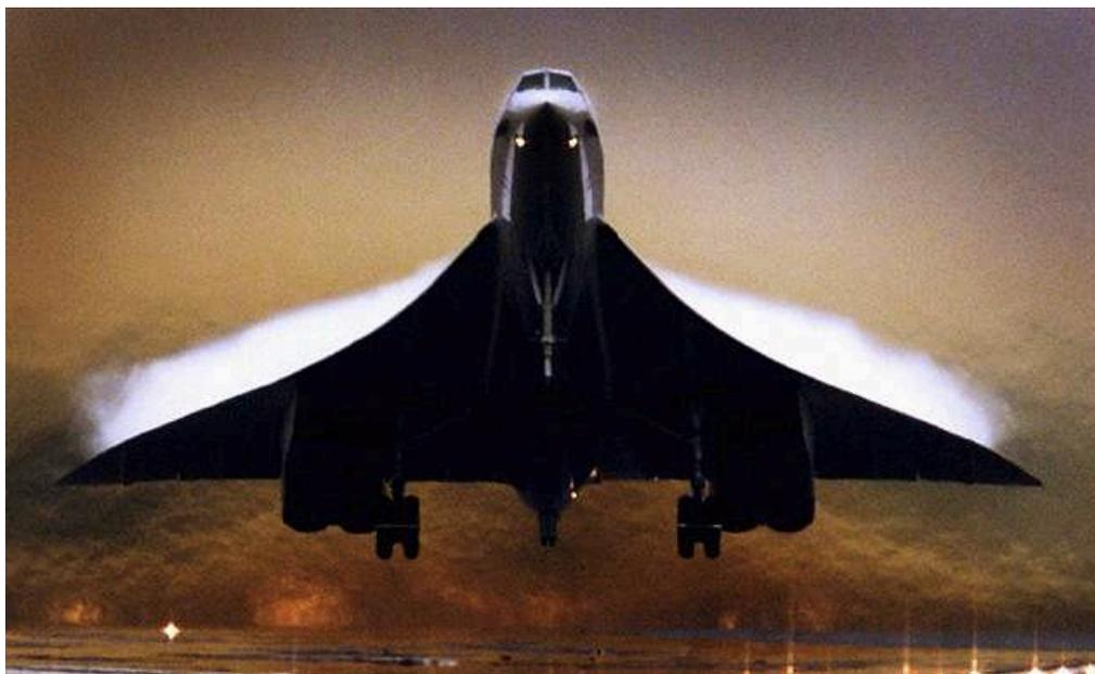
The low pressure formed by the Vortices over the wing are perfectly illustrated here, as well as the OGEE shape of the wing as in WG774 above.
